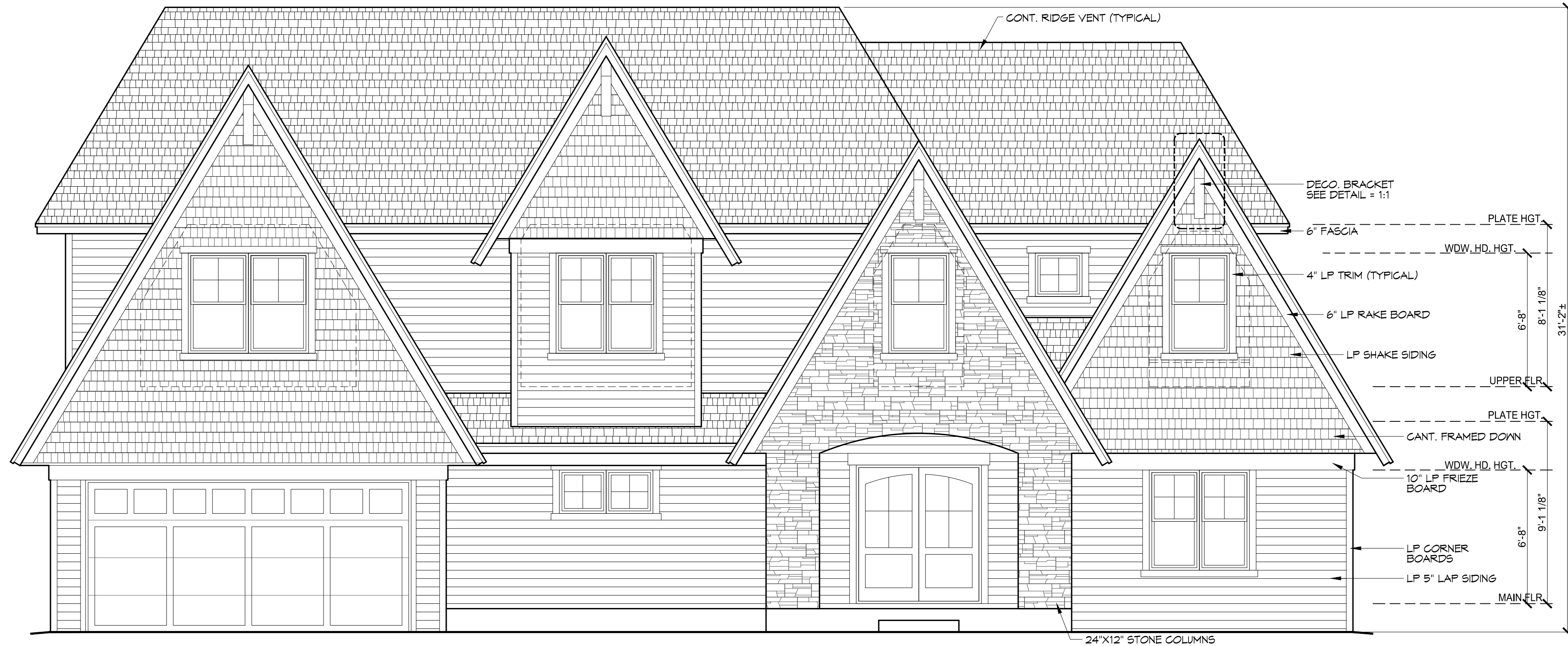
FRONT (NORTH) ELEVATION 1/4" = 1'-0"
